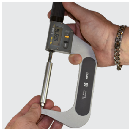
Length measurement of a lathed part
