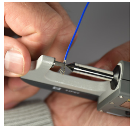
Cable crimping measurement
