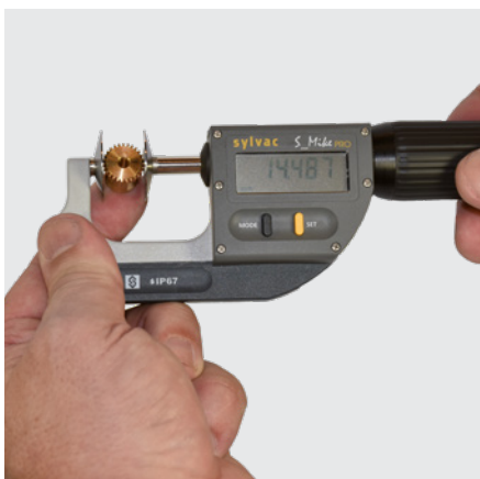
Part measurement with a S_Mike PRO Disk
