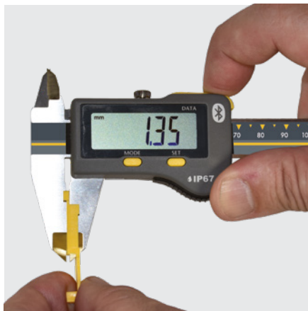
Part measurement with sending data
