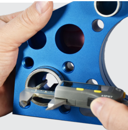
Deep measurement with S_Cal EVO Smart DM
