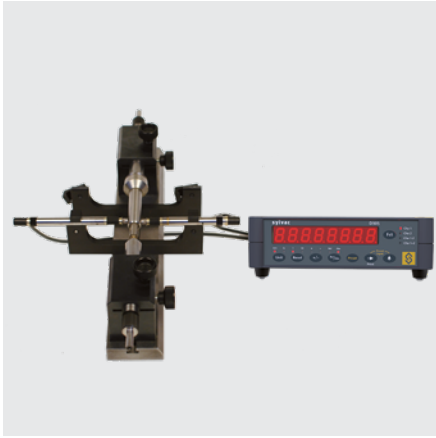
Measuring a shaft with 2 probes (A+B)
