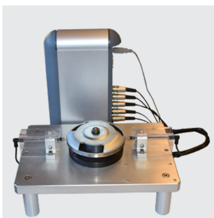
Capacitive probes connected to a D200S.
