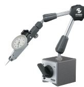
2220.10 with switch magnet (M)
