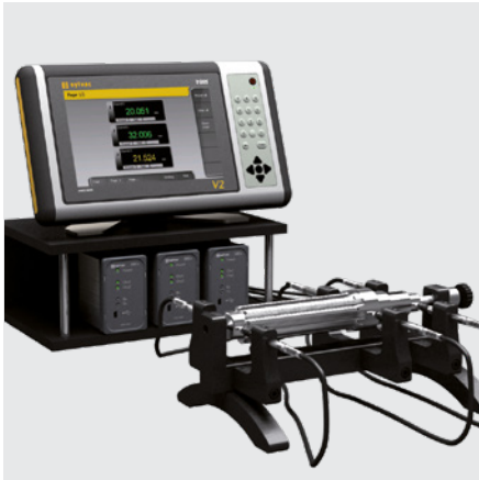
P5 probes connected to a D302 coupled with D300S for OD, concentricity and cylindricity measurements
