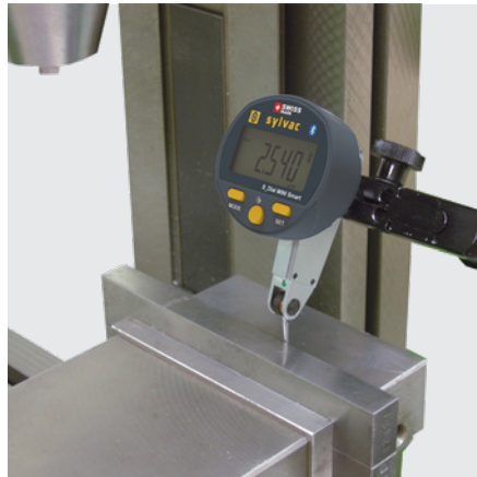
Checking the alignment on milling machine.
