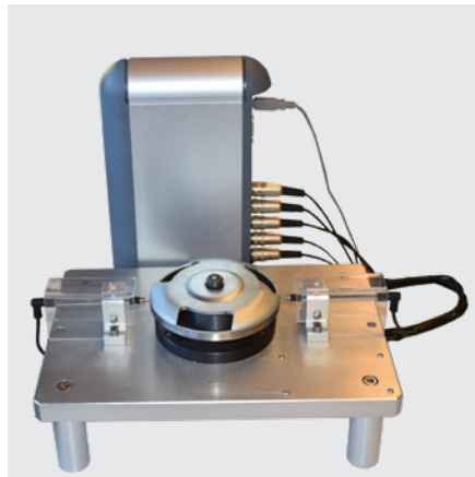
Capacitive probes connected to a D200S.
