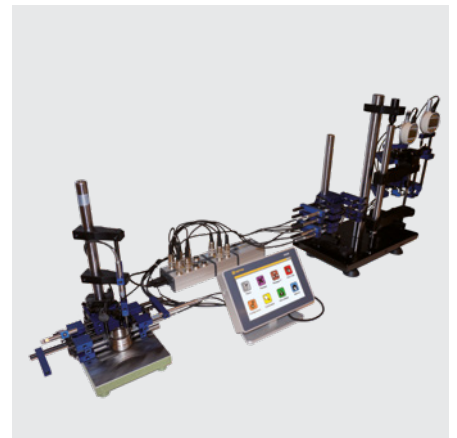
Probes and indicators connection through M-BUS inputs
