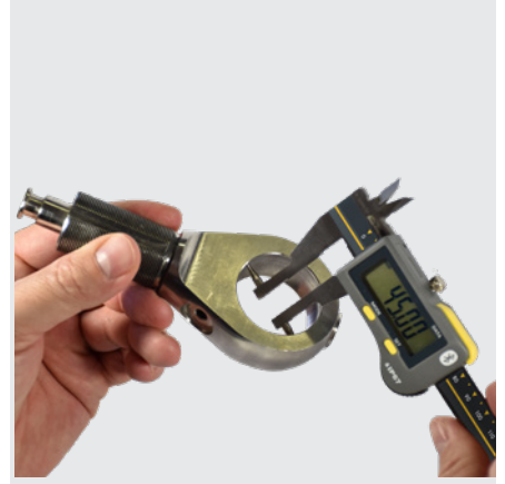
Internal measurement with S_Cal EVO Smart PJ
