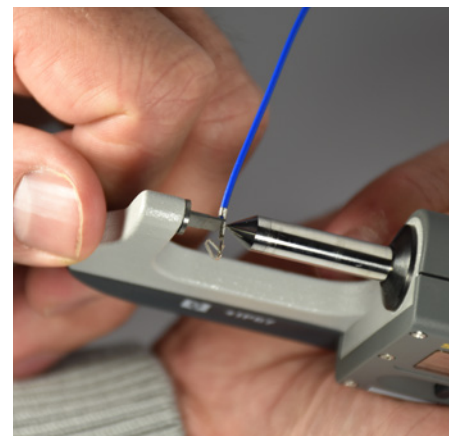
Cable crimping measurement
