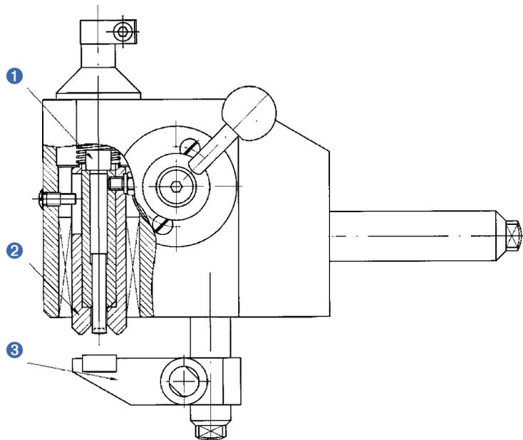
1 Messstift Measuring Pin 2 Prisma Prism 3 Unterer Messschenkel Lower measuring leg
