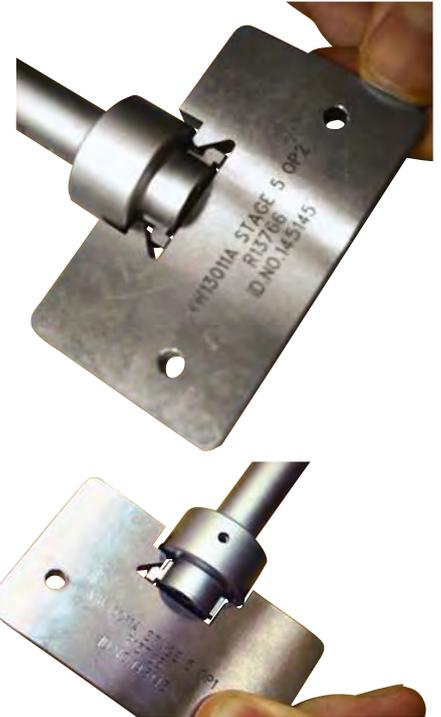
Single side measurement for set-up / symmetry
